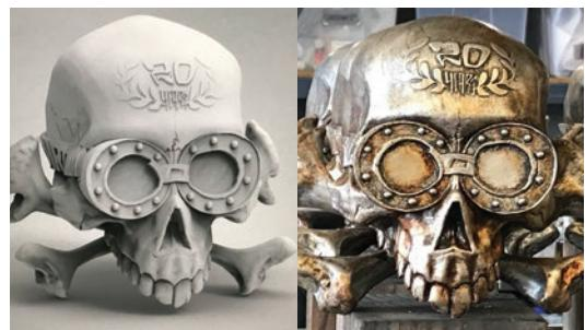
Thingergy's finishing process depends on the desired use. They primarily print in PLA filament, but also use ABS and TPU and occasionally PVA for dissolvable supports. Some prints are coated with Smooth-On's XTC before being body-shopped, primed, and painted. On other projects they body-shop and mold the prints, and then cast in other materials that are sometimes more flexible or durable.
